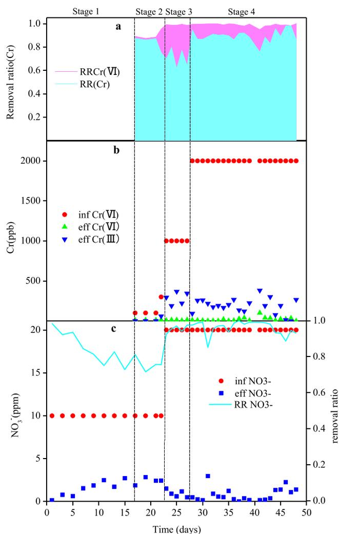
**Fig. 2.** (a) The total (Cr), Cr(VI) removal rate (RR); (b) concentrations of influent Cr (VI) (ppb), effluent Cr(VI) (ppb), and effluent Cr(III) (ppb); and (c) concentrations of influent NO<sub>3</sub>-N (ppm), effluent NO<sub>3</sub>-N (ppm), and NO<sub>3</sub>-N removal ratio in the MBfR.
