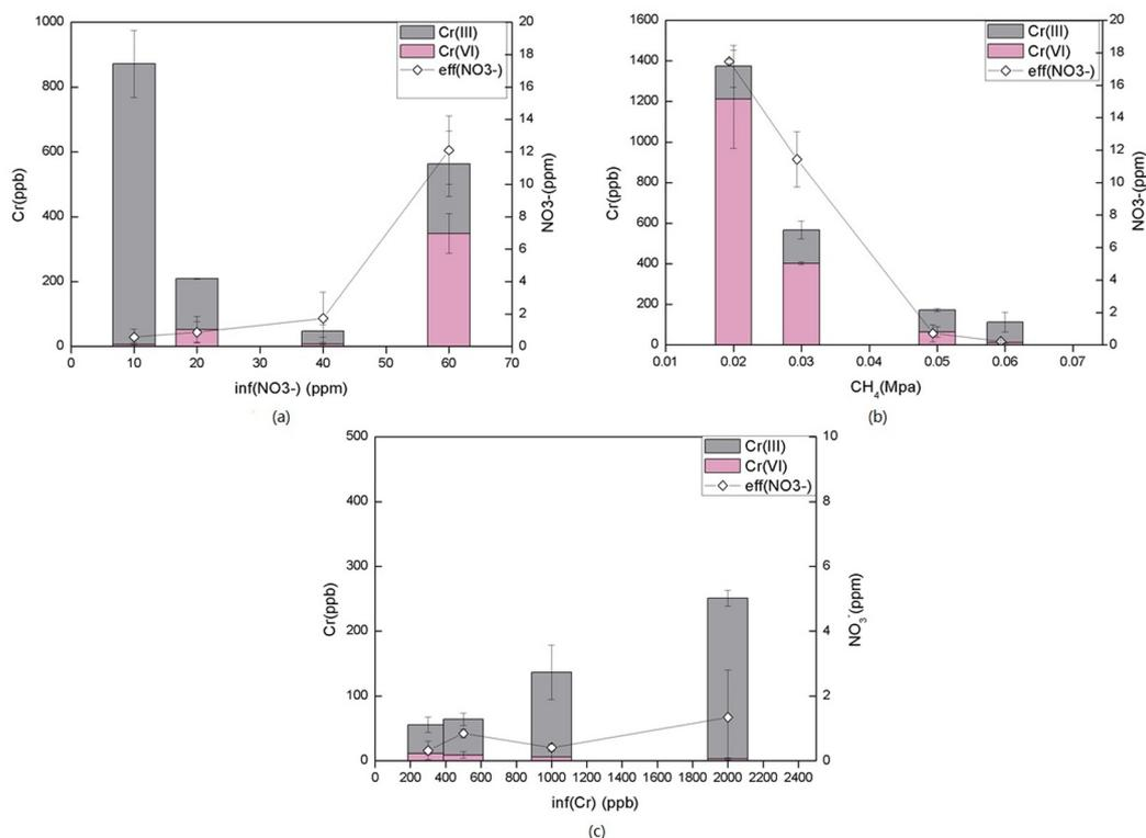
**Fig. 6.** The average concentrations of effluent NO<sub>3</sub><sup>-</sup> and Cr(VI)/Cr(III) at steady states of the short-term stages for (a) varied nitrate loadings; (b) varied CH<sub>4</sub> partial pressures; and (c) varied Cr(VI) loadings.
