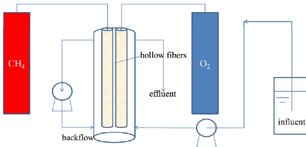
Fig. 1. A schematic of the bench-scale reactor used in the study.
