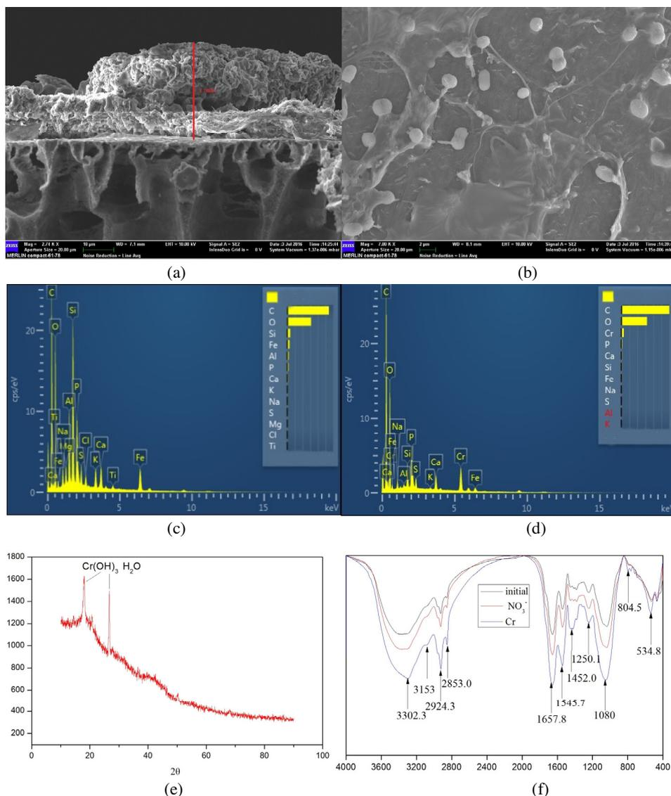
**Fig. 5.** (a) Scanning electron micrograph of section fiber; (b) surface biofilm from MBfR; (c) an EDX of the initial biofilm; (d) an EDS obtained from the insoluble precipitate formed in Cr(V)-reducing biofilm and the random area from reactor; (e) an XRD analysis of biofilm; (f) an FTIR analysis of the biofilm before and after the addition of NO<sub>3</sub><sup>-</sup> and Cr.
