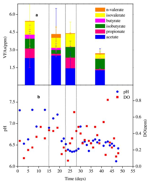
**Fig. 3.** (a) Average concentrations of VFA products in the four stages (ppm); (b) pH and DO in the MBfR during the four stages (ppm).
